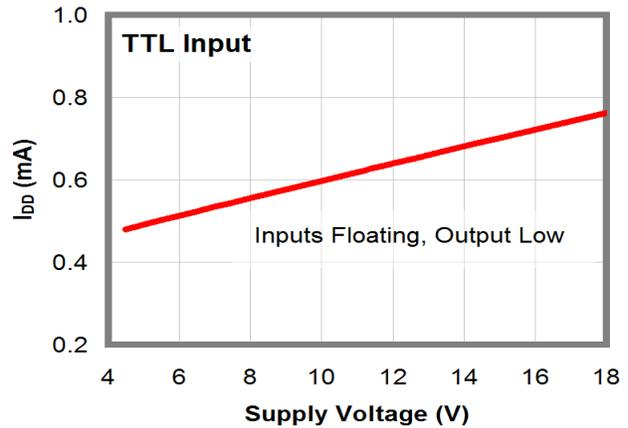
Figure 11. I<sub>DD</sub> (Static) vs. Supply Voltage (Note 13)
