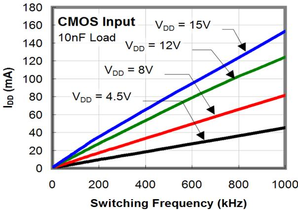
Figure 14. I<sub>DD</sub> (10 nF Load) vs. Frequency
