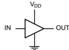
**Figure 51. Non-Inverting Driver**
