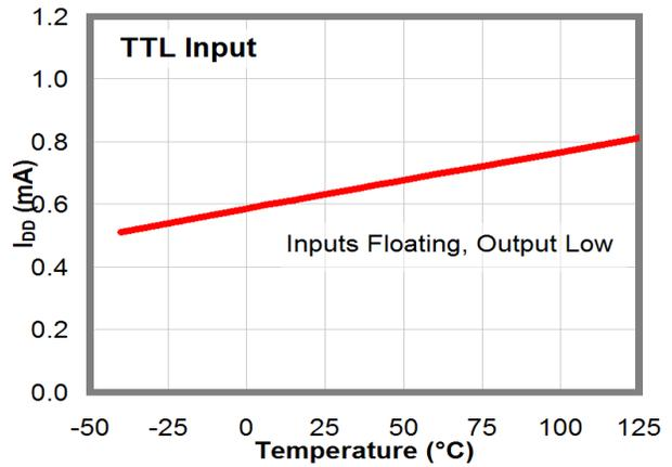
Figure 17.  $I_{DD}$  (Static) vs. Temperature (Note 13)
