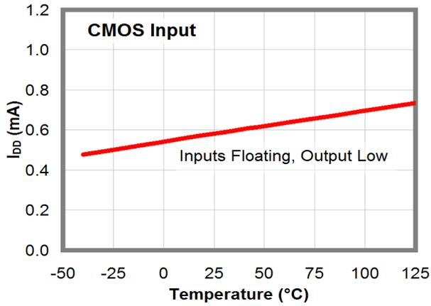
Figure 16.  $I_{DD}$  (Static) vs. Temperature (Note 13)
