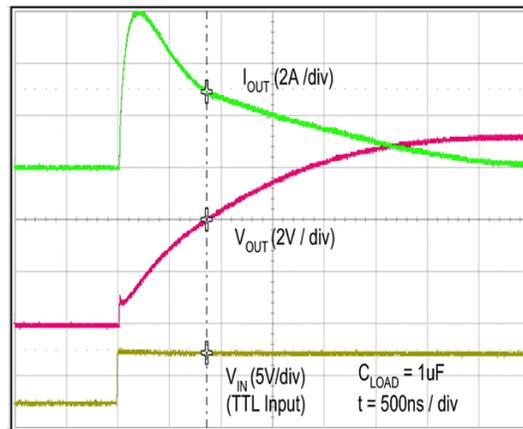
Figure 43. Quasi-Static Source Current with V<sub>DD</sub> = 8 V (Note 14)
