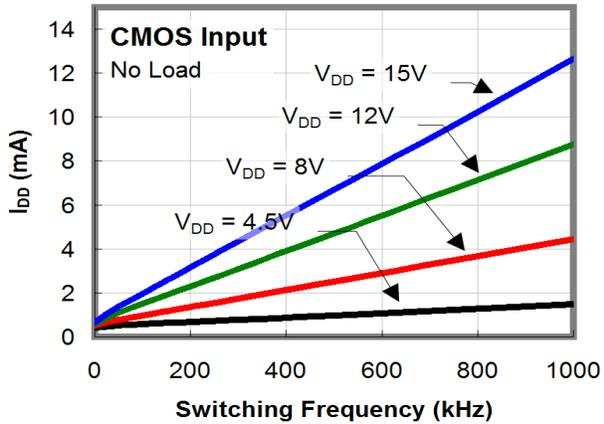
Figure 12. I<sub>DD</sub> (No-Load) vs. Frequency
