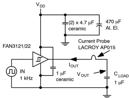
Figure 45. Quasi-Static I<sub>OUT</sub> / V<sub>OUT</sub> Test Circuit
