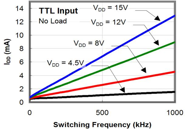
Figure 13. I<sub>DD</sub> (No-Load) vs. Frequency
