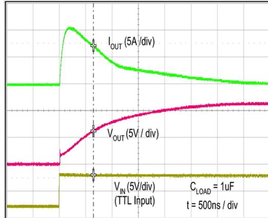
Figure 41. Quasi-Static Source Current with V<sub>DD</sub> = 12 V (Note 14)
