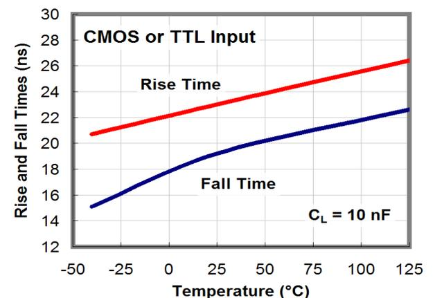
Figure 39. Rise and Fall Time vs. Temperature
