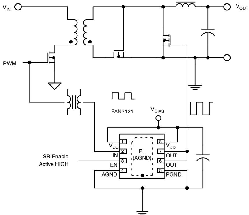
Figure 54. Hybrid Synchronous Rectification in a Forward Converter
