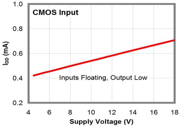
Figure 10. I<sub>DD</sub> (Static) vs. Supply Voltage (Note 13)
