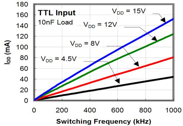
Figure 15. I<sub>DD</sub> (10 nF Load) vs. Frequency
