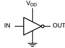
**Figure 49. Inverting Configuration**
