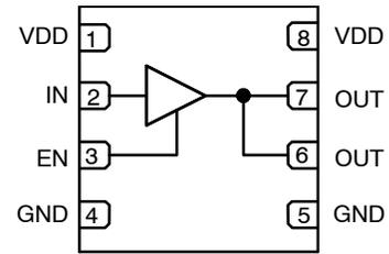
Figure 2. FAN3122 Pin Configuration
