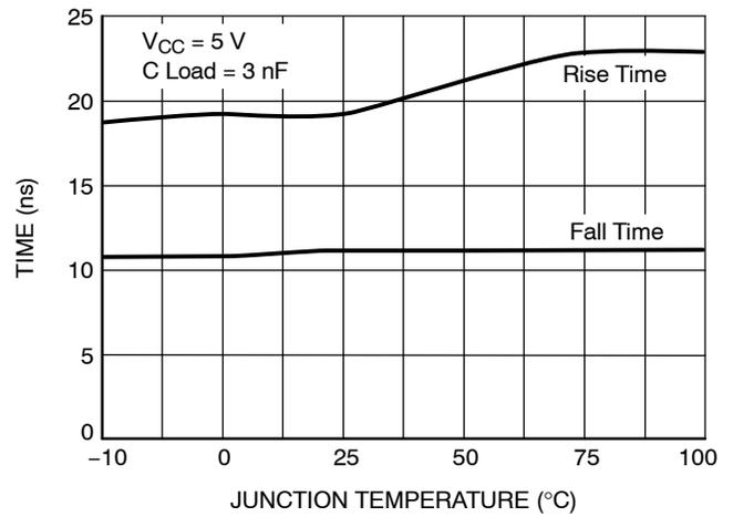
Figure 10. DRVL Rise and Fall Times vs. Temperature
