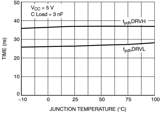
Figure 13. DRVH and DRVL  $t_{pdH}$  vs. Temperature
