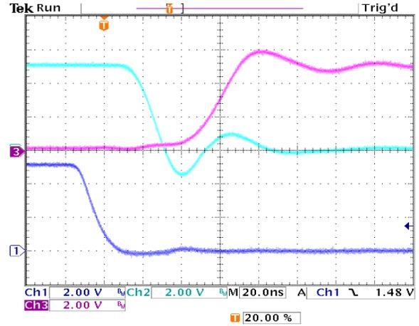
Figure 8. DRVH Fall and DRVL Rise Times
