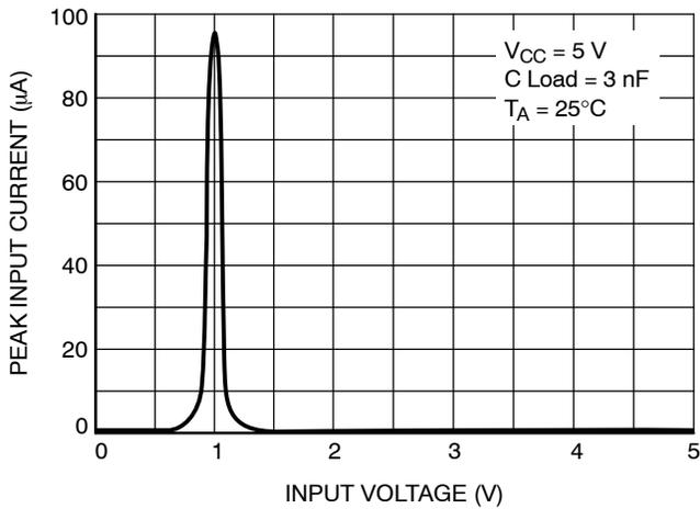
Figure 15. IN Pin Input Current vs. Input Voltage
