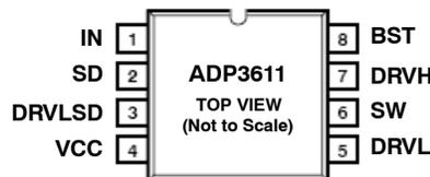
Figure 6. 8-Lead DFN 2 x 2 mm Package
