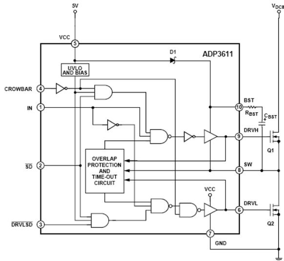
Figure 18. Detailed Block Diagram of the ADP3611
