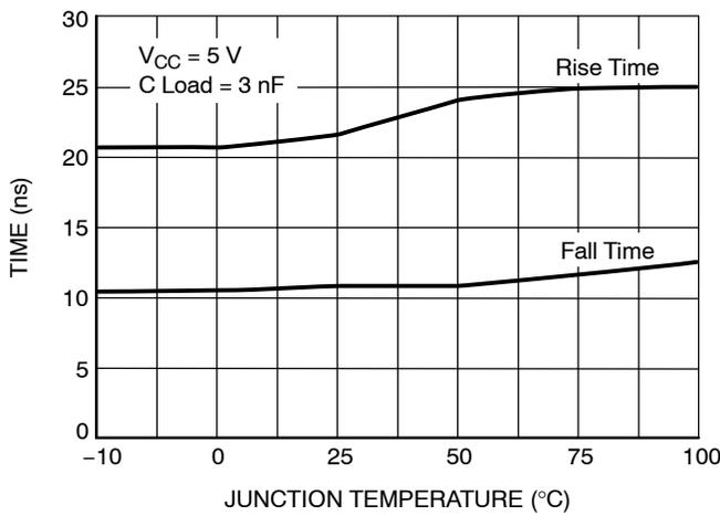
Figure 9. DRVH Rise and Fall Times vs. Temperature
