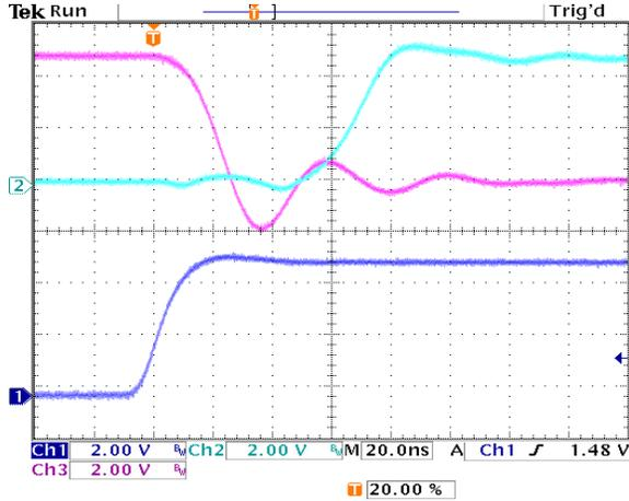
Figure 7. DRVH Rise and DRVL Fall Times
