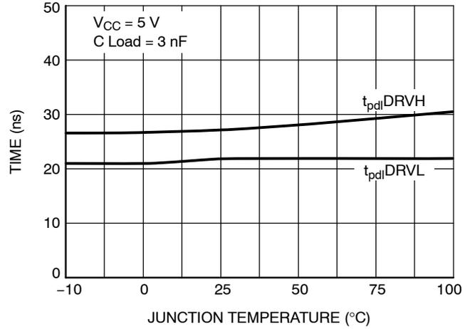
Figure 14. DRVH and DRVL  $t_{pdL}$  vs. Temperature
